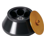
NA-11 250ml × 6 (tubes): 12,000rpm:22,540G
