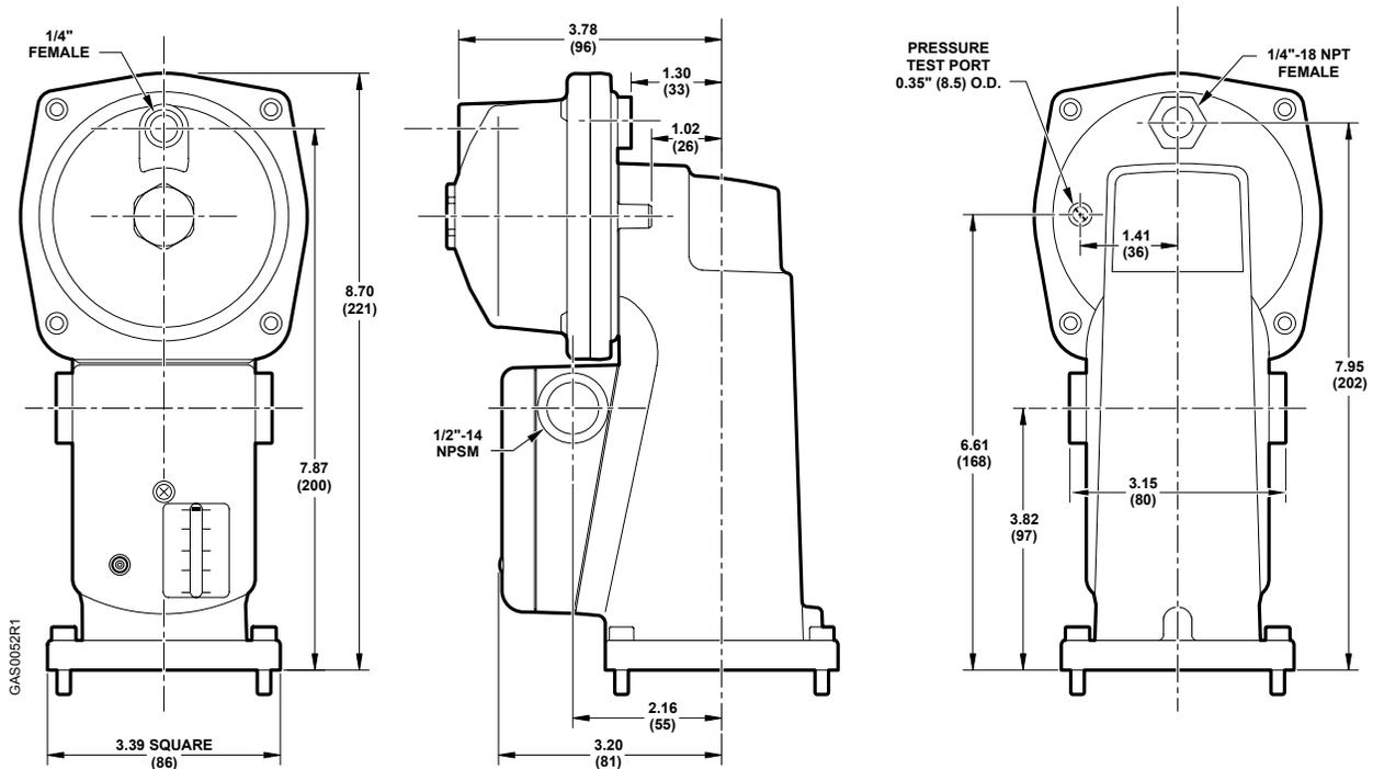
**Figure 3. SKP25...U.. Dimensions in Inches, Millimeters in Parentheses.**
