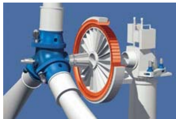
Figure 5: Gearless wind turbine (Picture by Enercon)
