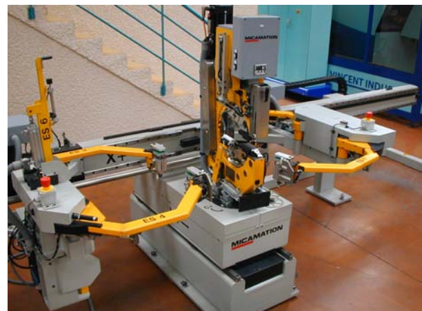
Figure 6: Taping machine MI 135 for flat coil technology
